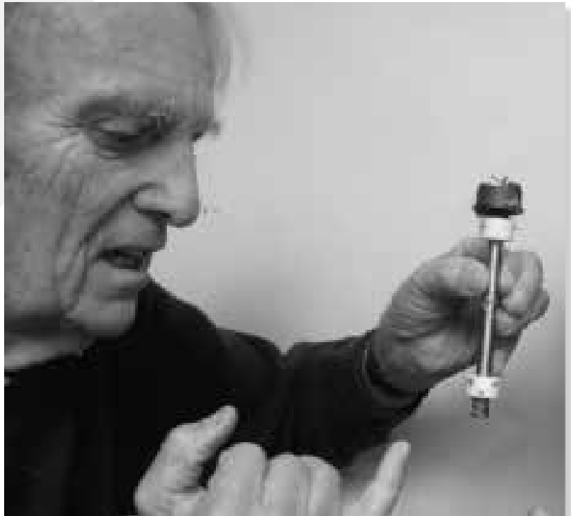
Sir Martin Wood with the mixing chamber of the first commercial dilution refrigerator, built at Oxford Instruments
