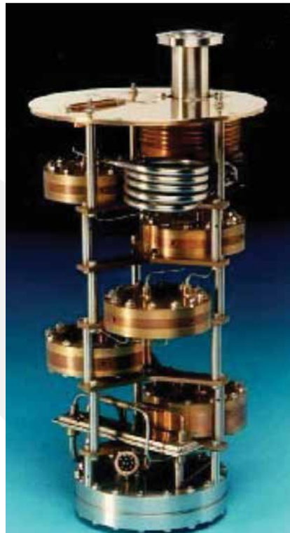
Early 70's dilution unit with copper heat exchanger
